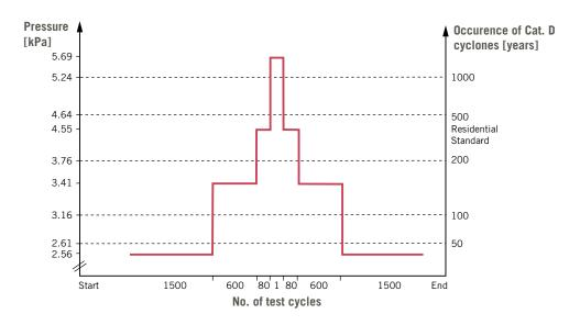
The test design consists of repeated test cycles of wind pressure.
